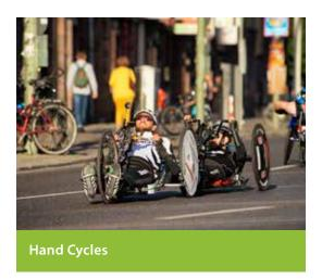
**Hand Cycles**. A handcycle is a type of bicycle that is propelled by the arms rather than the legs. Most hand cycles are tricycle in form, with two coasting rear wheels and one steerable powered front wheel. Despite usually having three wheels, they are also known as hand bikes.
