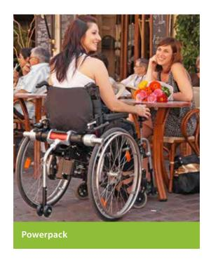
Powerpacks. The Powerpack is a two-wheeled power pack that converts a manual wheelchair into a powered chair. Manually wheeling over surfaces that are not smooth can be exremely effortful. Converting a manual chair to a powered chair can assist manual wheelchair users to access more trails for longer periods. The power pack is controlled with a handheld remote. Movement of the chair is operated by pressing the power button.
